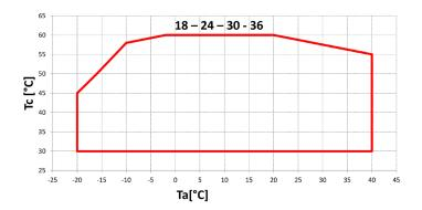
Ta: external air temperatureTe: evaporating temperatureTe: condensing temperature
