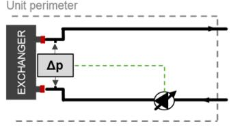
Flowzer VDE requires a differential pressure transducer to be installed in the machine. Through this transducer, the inverter can gauge the actual pressure at the ends of the heat exchanger installed in the machine and it can automatically adapt the pump speed for a constant flow value under all conditions. Flowzer VDE must be combined with Flowzer VP.
