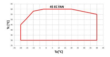
Ta: external air temperatureTe: evaporating temperatureTe: condensing temperature
