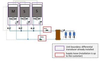
The HYZER E VPS with TD-based control function combines the Multilogic function, which is used to manage multi-machine systems, with the FLOWZER VPS with DT-based control control for variable flow systems.
